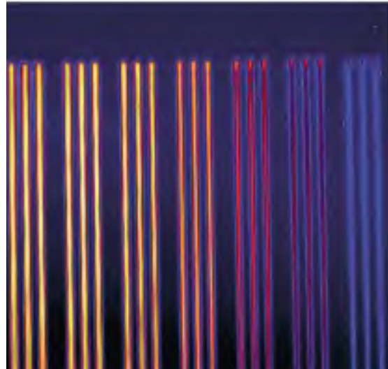
Fig. 1: Emission SRI image of groups of three identical LCE grooves, each group produced with a different laser power. Lighter colours indicate higher local doping levels. Local high doping can be achieved by using etching chemicals containing phosphorus in LCE with varying laser energy values. Depending on the choice of parameters, we have already measured sheet resistance values between 15 and 40 \Omega/\text{sq} . In comparison to fig. 2, the doping can be clearly attributed to the etching fluid containing phosphorus.
