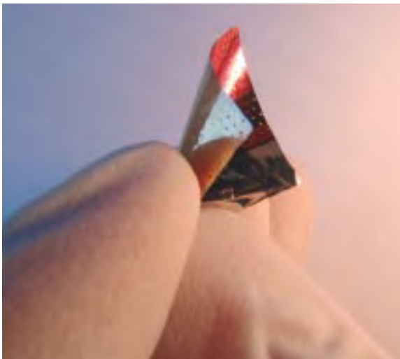
Fig. 3: Organic solar cell on a flexible substrate with contacts through perforations. Electrical connection of the solar cell via holes allows inexpensive transparent electrodes with low sheet conductivity to be used. This solar cell concept combines the demands for inexpensive materials and efficient production technology applying roll-to-roll processes.
