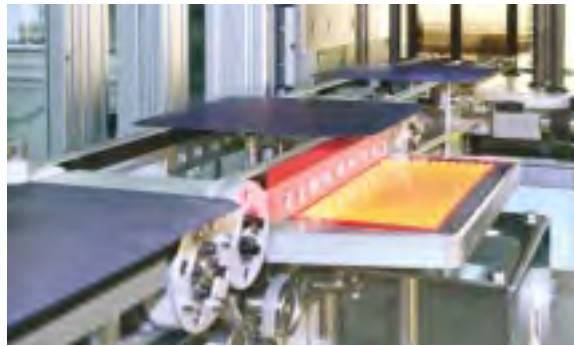
Fig. 2: Various high-resolution measurements can be carried out in the PV-TEC characterisation laboratory. The most important types of measurement are: infra-red multi-functional measurement, large-area determination of the external quantum efficiency, spatially resolved lifetime measurement, sheet and contact resistance topography, reflectance spectroscopy. In-line measurement instruments are integrated into the processing facilities.
