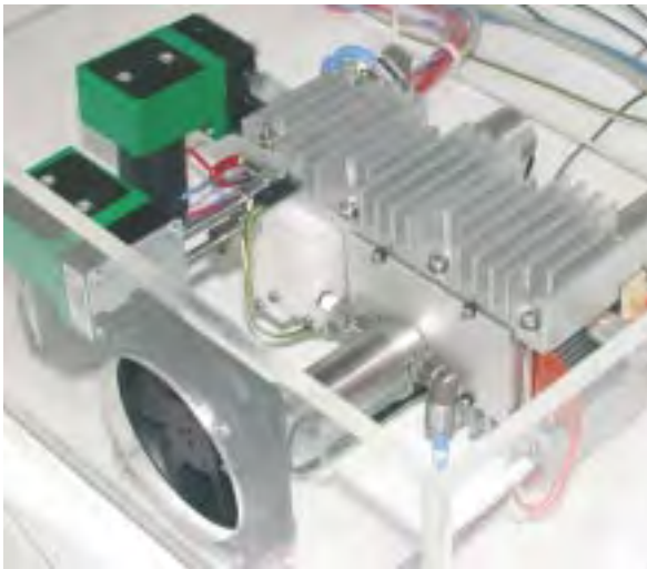
Fig. 1: The photo shows a portable fuel cell system, which was housed in transparent PMMA for demonstration purposes. The fuel cell stack with its cooling fins and the peripheral system components, pumps and fans, are clearly visible.
