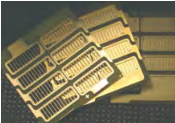
Fig. 1: Planar fuel cells can be integrated into the housing of devices and can be operated passively, i.e. without ventilators or pumps. We use inexpensive circuit boards and polymer materials with channel structures which we coat by individually optimised processes. Eight single cells are connected in series within one plane. This results in a higher voltage which is adapted to the specific load.
