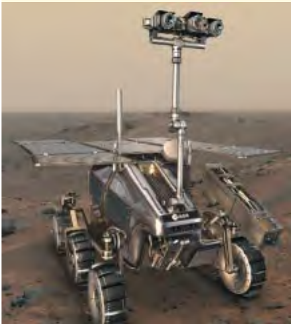
Fig. 1: ExoMars is a planned European Mars-Rover, which should be started in 2013 from the Kourou Spaceport as part of the Aurora Programme. Electricity for the rover, which weighs about 190 kg, is generated by III-V multi-junction solar cells.
