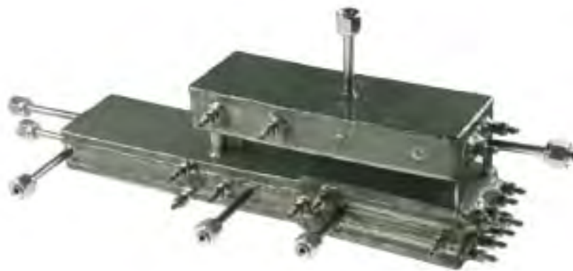
Fig. 3: High-temperature unit. The evaporator and superheater can be seen to the left. The actual steam reforming reactor is connected at the lower right. Above it is the two-stage shift reactor. The various pipe connectors serve as inlets and outlets for the various reactants and products, and also for connecting temperature sensors.
