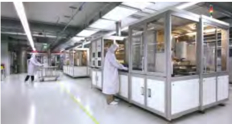
Fig. 1: Extremely modern production facilities are available in PV-TEC. The basic equipment includes: Multi-functional wet-chemical batch-processing facility, in-line texturing system, tube diffusion/oxidation, plasma-enhanced chemical vapour deposition (PECVD), sputtering equipment, screen-printing line, laser system, solar cell tester and solar cell sorter. High-speed, in-line measurement instruments are integrated into the equipment.
