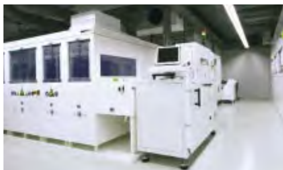
Fig. 4: The wet-chemical cluster consists of in-line and batch-processing multi-purpose systems, as well as a chemicals supply module. Innovative functions such as single-sided etching are included as well as the standard etching processes for monocrystalline and multicrystalline silicon. The accompanying analytical methods include titration, chromatography, infrared and ultraviolet spectroscopy.
