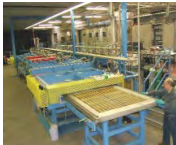
Fig. 3: Sputtering equipment to coat steel pipes with absorber coatings and glass panes with reflective coatings.
