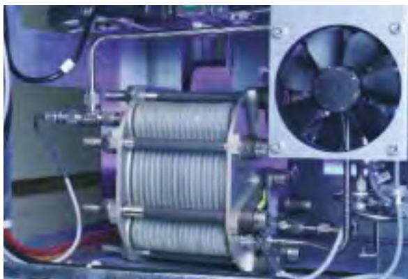
Fig. 2: Cell stack for the pressure electrolyser, in which the distribution structures are made cost-effectively out of polymer materials. The stack consists of 15 single cells.
