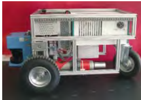
Fig. 2: Together with Fraunhofer IAIS, we are developing a fuel-cell power supply for the robotics platform, "VolksBot RT". The photo shows a three-wheeled version (w x h x d: 540 x 410 x 630 mm 3 ), in which the fuel cell has already been integrated. The laser scanner in the blue unit at the front is used for navigation purposes.
