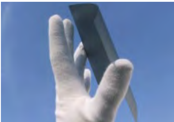
Fig. 1: Using different wire pitches on the wire-guiding rollers, we have succeeded in producing neighbouring wafers with varying thicknesses. It was then possible to cut wafers with thicknesses between 140 and 250 µm, e.g. for tests of solar cell concepts on multi-crystalline material. In the graph, the measured average wafer thicknesses are plotted as a function of the wafer position on the wire-guiding rollers. The intended wafer thicknesses, which are indicated by the solid line, were achieved nearly in all cases.
