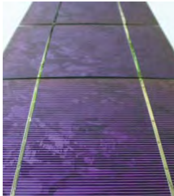
Fig. 1: Laser-soldered cell string with 156 mm cells from the PV-TEC production line.
