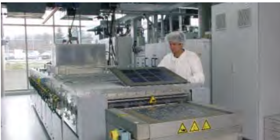
Fig. 1: Sputtering system for in-line deposition of aluminium and silicon nitride.
