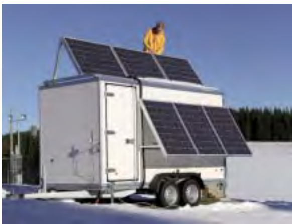
Fig. 3: "EVEREST" Maxibox, consisting of a photovoltaic system (960 Wp) on the roof and the side of the trailer, and a direct methanol fuel cell (325 W) and batteries with a capacity of 1320 Ah inside. To transport the measurement system (fig. 2) for mobile applications, the Maxibox is constructed on a trailer.
