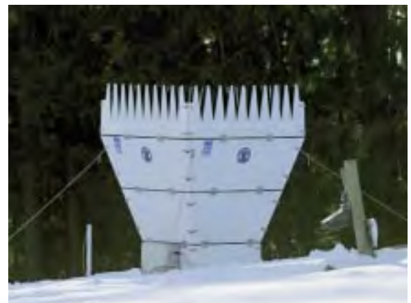
Fig. 2: "Doppler-Sodar-Messsystem PCS.2000-24" from the Metek company. This mobile measurement station draws its power from the "EVEREST" Maxibox (fig. 3).
