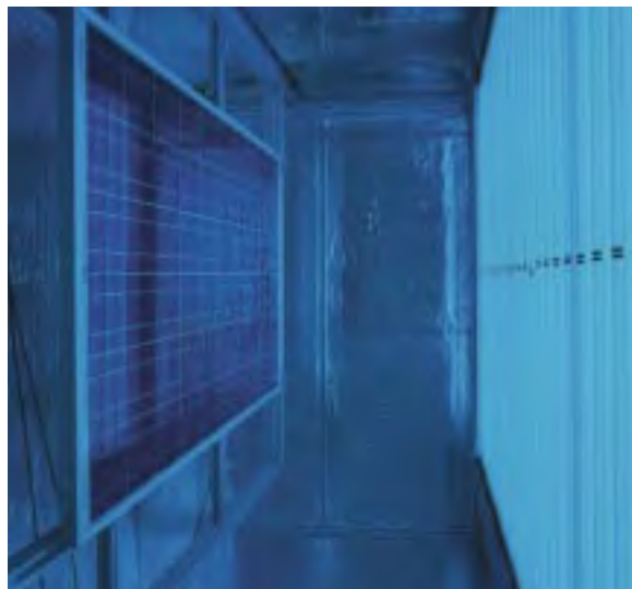
Fig. 1: UV test stand for photovoltaic modules with dimensions up to 1.4 x 2.4 m 2 .
