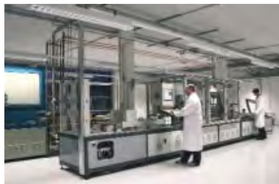
Fig. 2: Prototype production unit for photovoltaic modules with the tabber-stringer (in the foreground) and the laminator (left).
