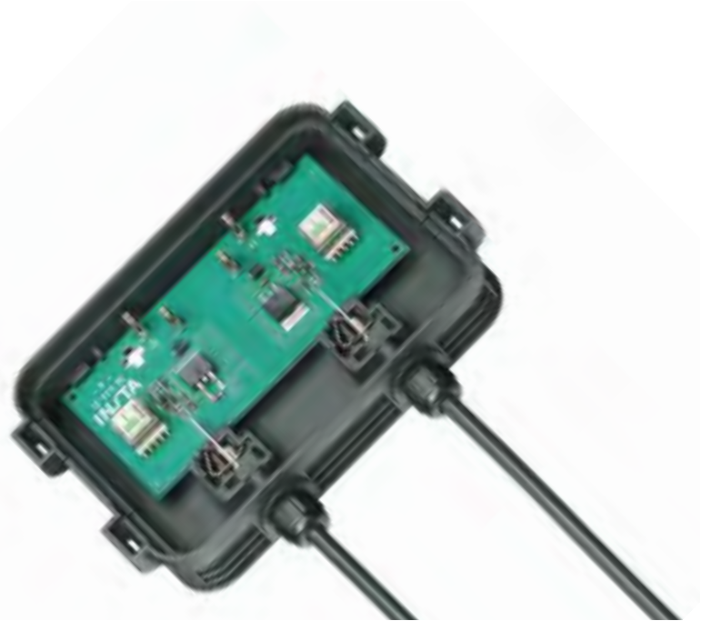
Fig. 1: DIODLESS connection circuit without diodes with a rated current of 16 A, for two sub-groups of solar cells. Our industrial partner plans the development of a complete family of connection circuits without diodes which apply the new concept.
