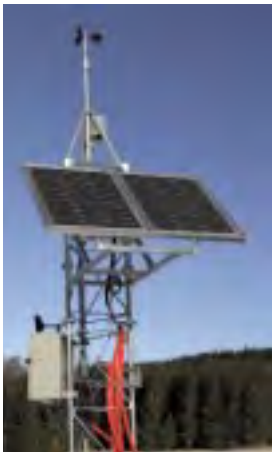
Fig. 1: Stand-alone wind measurement system, "Meteo-32" with the "Wicom" data logger from the Ammonit company (left). The power for this measurement station is supplied by the "EVEREST" Minibox (right), consisting of a photovoltaic generator with a power of 100 Wp, a direct methanol fuel cell with a power of 65 W and batteries with a capacity of 660 Ah.
