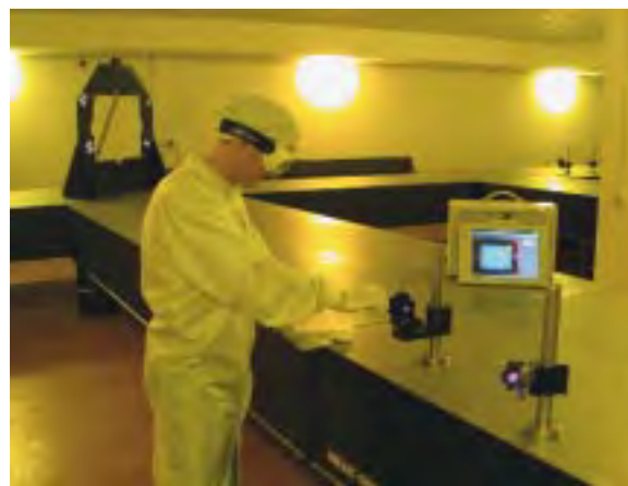
Fig. 2: The interference lithography laboratory at Fraunhofer ISE. Homogeneous grating structures can be generated here over areas of up to 1.2 x 1.2 m 2 .
