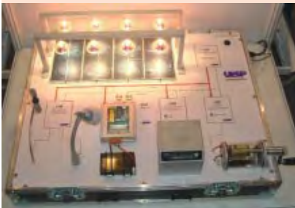
Fig. 1: This demonstration case shows a fully functional PV hybrid system with the Universal Energy Supply Protocol UESP. The individual components are connected with each other via a CAN bus and carry out the cost-optimised energy management with a standardised, manufacturer-independent protocol.
