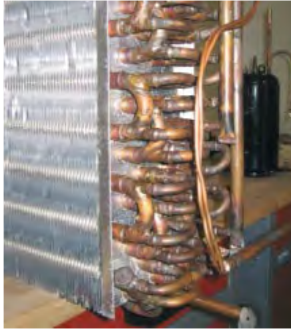
Fig. 1: With this newly developed combined evaporator 1 , two heat sources, such as exhaust air and solar energy, can be used simultaneously by the heat pump, without the cooler loop design becoming more complex. The refrigerant in the gap between the coaxial pipes can extract heat simultaneously from the liquid in the inner pipe and from the air current in the outer pipe. 1 Patent application by Fraunhofer ISE
