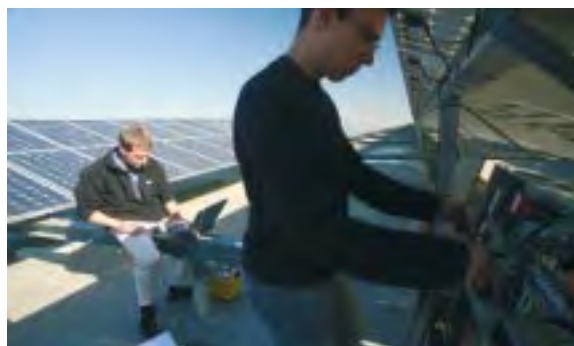
Fig. 2: Fraunhofer ISE experts during performance measurement of the 3 MW system located on the roof of the BMW factory in Dingolfing.
